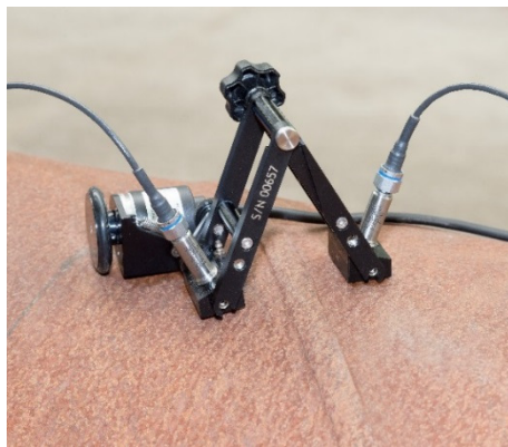
Weld inspection with TOFD scanner
